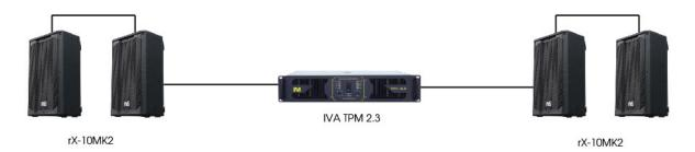
Compatible for 1 unit or 2 unit of rX-10MK2 each side.
