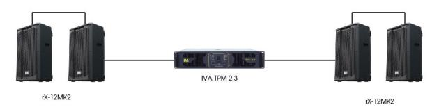
Compatible for 1 unit or 2 unit of rX-12MK2 each side.
